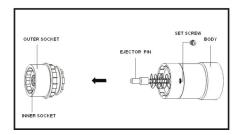
2) Prepare the inner and outer sockets which are suitable for the bolt to be fasten. First tighten the first set-screw incompletely, then tighten the second set-screw completely, third back to the first set-screw then tighten completely.
